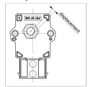
Lateral magnet offset will cause additional linearity error. The angle error, which is caused by radial displacement of sensor and position marker depends on the used position marker or magnet.
