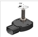
When the marking of the position marker points towards the connector, the sensor is near the electrical center position.
