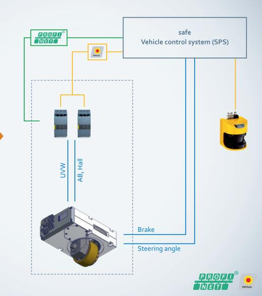
Integration of ArgoDrive into an AGV Use case SIMOVE by Siemens
