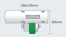
Wheel diameter 145mm 1,5m/s | 500kg Ground clearance 128mm
