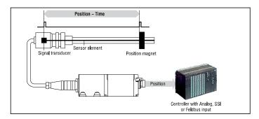
**Temposonics® RD4** the extremely robust sensor, ideal for continuous operation under harshest industrial conditions is completely modular in mechanic and electronic design. A rod-shaped sensor housing protects the sensing element. The sensor head accommodates the complete modulare electronic interface with active signal conditioning. Double encapsulation ensures high operation safety and optimum EMC protection.
