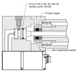
Minimum installation dimensions for magnetizable material
