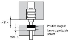
Bore in cylinder Ø 13...17 mm to push single wires with flat connector through.
