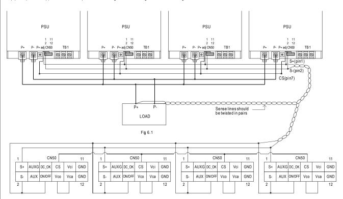
Note : In parallel connection, maybe only one unit (master) operate if the total output load is less than 5% of rated load condition. The other PSUs (slaves) may go into standby mode and their output LEDs will not turn on.
