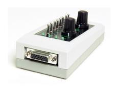
adjustment of velocity, positioning, torque etc. The signal is connected to AIN at MAC and MISxQ/R/S/T motors and at IO3 at MISxA/K motors.
