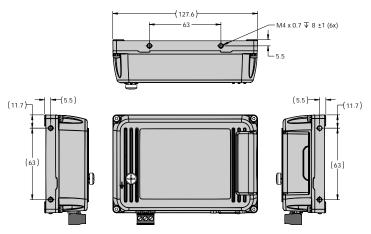
The BoX2 pro can be used as a bench top device or clipped onto a DIN rail. For custom mounting, the DIN rail mount can be moved from the standard position, opposite the connection, to a side. The mount can be removed for access to all the mounting points shown above.
