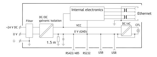
The operator panel has galvanic isolation against the 24 V DC power supply but no galvanic isolation between the communication ports for RS-232, RS-422/RS-485 and USB. Only the Ethernet connection has galvanic isolation.
