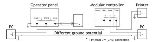
When a PC is connected to the operator panel, the internal 0 V (GND) of the panel is connected to the protective ground via the PC.
