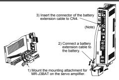
Note. Be careful not to catch battery extension cable on peripheral equipment or by your fingers. Doing so may cause a disconnection of the CN4 connector due to stress on the connector connection part.
