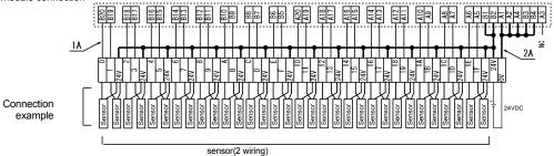
(2) When the sink output module connection
