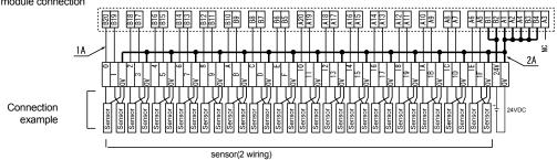
(2) When the source output module connection
