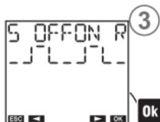
Turning on at sunset, turning off during the night, turning on during the night, turning off at sunrise.
