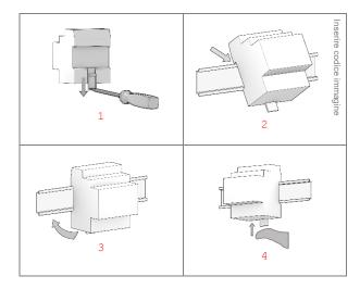
To unmount the device, make sure to unplug the network connection and the bus terminal from its housing. Use a screwdriver to slide down the lock and remove the device from the rail.
