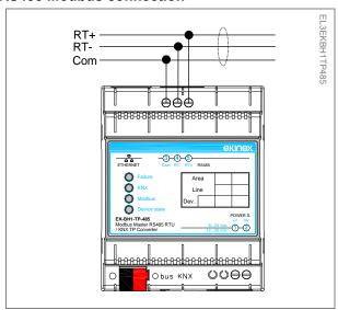
In order to terminate the RS485 network and balance the line impedance, you must enter the terminating resistor (120  $\Omega$ ), by setting ON the 1-way microswitch B.
