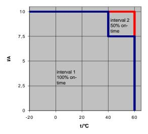
For the duration of on-time only the charge and discharge cycles are relevant. If the buffer-module is charged and works in the standby-mode there is no heating of the unit. From the thermal point of view this can be compared with a switched-off unit.
