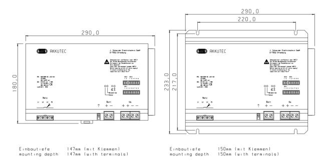
To attach the AKKUTEC module directly on the mounting plate you can purchase optional mounting flanges.
