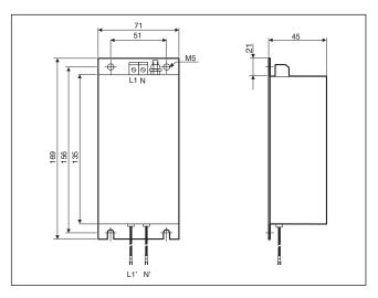
Filter type MF-3F480-010.230, MF-3F480-025.230 and MF-3F230-050.230
