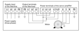
All cables must be shielded and earthed at both ends in order to reduce cable radiation. Earth motor, bond to filters. Position and environment of the filter unit should be the same as for the servo amplifier, as specified in the MR-J2S instruction manual.
