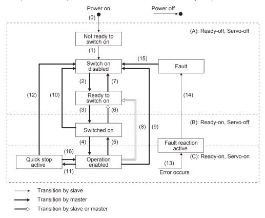
When the communication state is "IDLE", the state will always be Switch on disabled.
