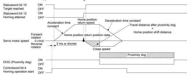
Note. After the front end of the proximity dog is detected, if the rear end of the proximity dog is detected without reaching the creep speed, [AL. 90] occurs. Check the length of the proximity dog or check the home position return speed and creep speed.
