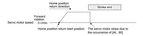
When the stroke end is detected
