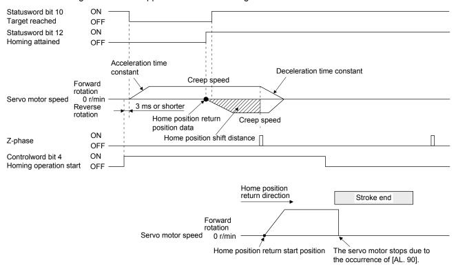
When the stroke end is detected
