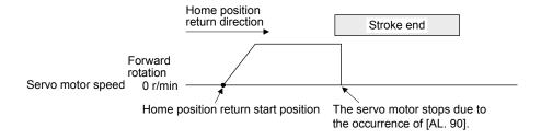
When the stroke end is detected
