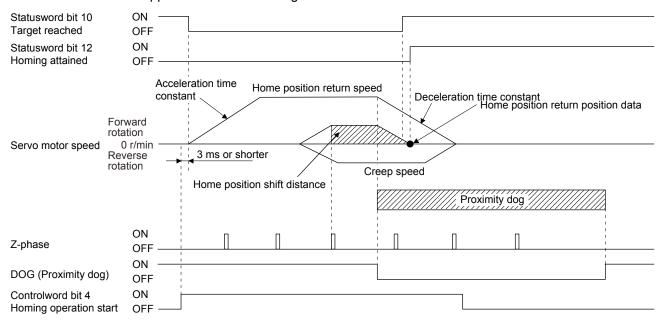
Note. After the front end of the proximity dog is detected, if the rear end of the proximity dog is detected without stop, [AL. 90] occurs. Check the length of the proximity dog or check the home position return speed and creep speed.
