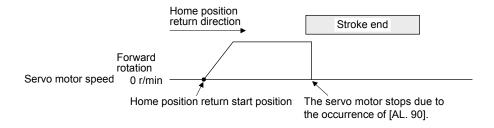
When the stroke end is detected
