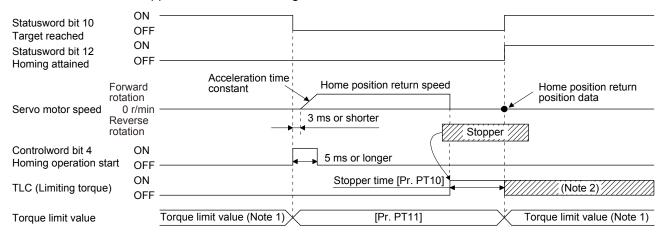
Note 1. When Method -4 is set, the torque limit value of Positive torque limit value (P24800) is applied. When Method -36 is set, the torque limit value of Negative torque limit value (P24801) is applied.
