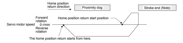
Note. The software limit cannot be used with these functions.
