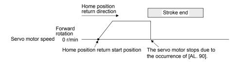
When the stroke end is detected
