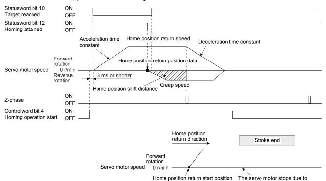
When the stroke end is detected
