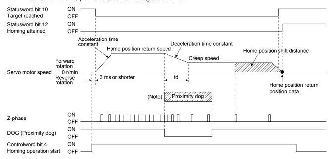
Note. After the front end of the proximity dog is detected, if the distance after proximity dog is traveled without reaching the creep speed, [AL. 90] occurs. Set the travel distance after proximity dog enough for deceleration from the home position return speed to the creep speed.
