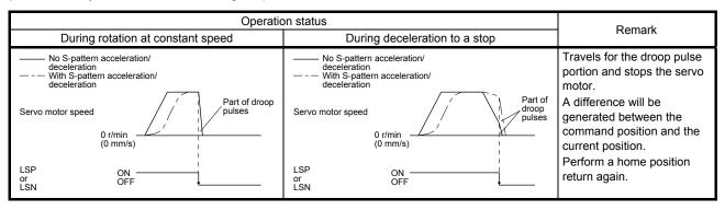
Perform a return as follows when the stroke end is detected.
