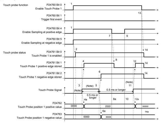
Note. Turn on and off Touch Probe Signal so that both the on time and off time are 0.5 ms or longer.
