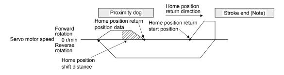
Note. The software limit cannot be used with these functions.
